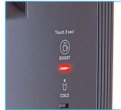
Hot water booster button to raise the temperature from 90° C to 95° C (Limited quantity)
